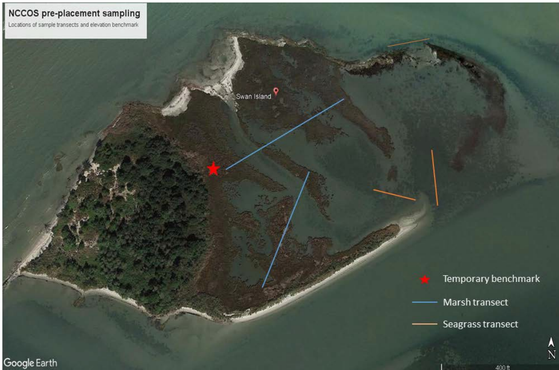
Figure 3. Satellite image of Swan Island indicating the location of the temporary benchmark and the marsh and seagrass transects surveyed in August 2018, prior to restoration of the islands natural features with the placement of dredged sediments.
