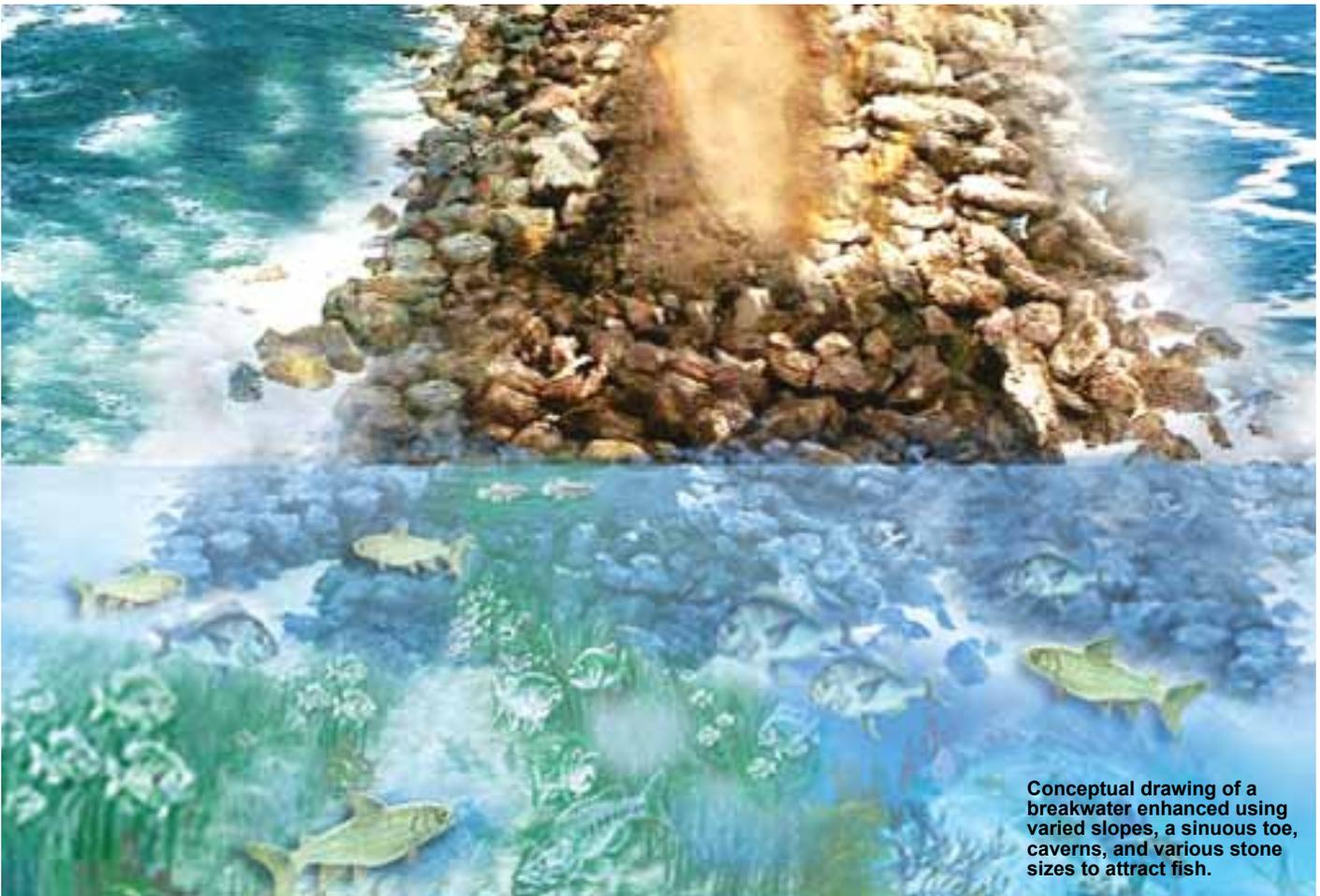
Conceptual drawing of a breakwater enhanced using varied slopes, a sinuous toe, caverns, and various stone sizes to attract fish.
