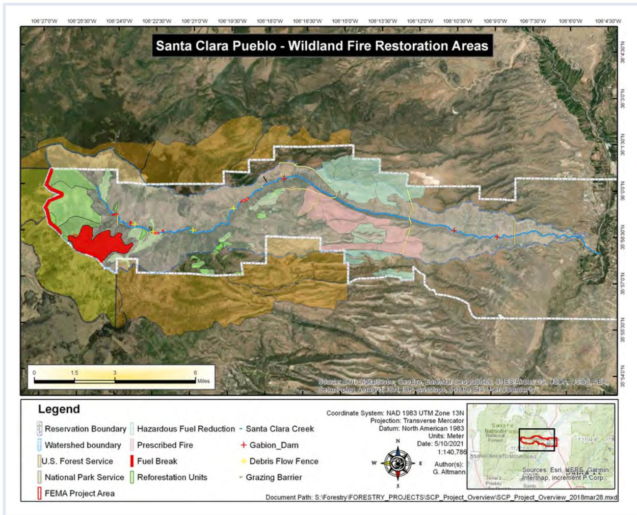
FIGURE 1 Locations within the Santa Clara Canyon where natural infrastructure materials were installed to manage post-wildfire erosion
