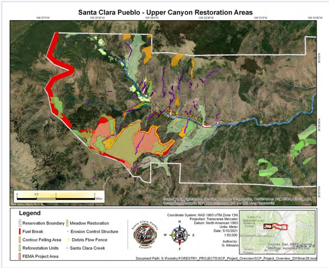
FIGURE 4 Locations where natural infrastructure materials were installed as erosion control features in the Upper Reach of the Santa Clara watershed
